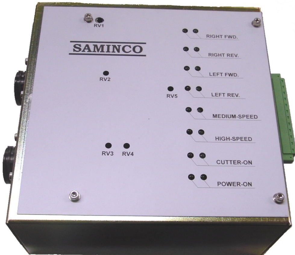
Continuous Miner Interface Box with Cutter Head Feedback
