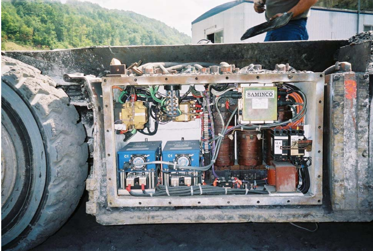
Typical Saminco JS-400 Shuttlecar panel
