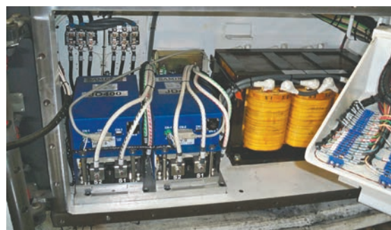
Two drive system for continuous miners
