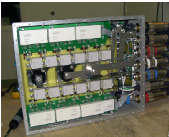
Fig. 7: The inverter package shown in Fig. 6, with the top cover removed. The connecting cables are visible on the far right. Courtesy of Saminco, Inc.
