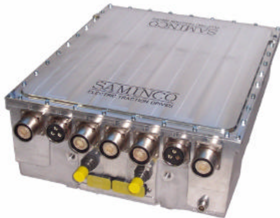
Fig. 6: 220 KW water cooled inverter drive for hybrid buses, using induction motor. Control and signal connection is at the bottom (square covers). The cooling water is supplied through the two yellow connectors. On the top are three motor connectors, two (black) connectors for external braking resistor and two connectors for \pm DC link. Courtesy of Saminco, Inc.
