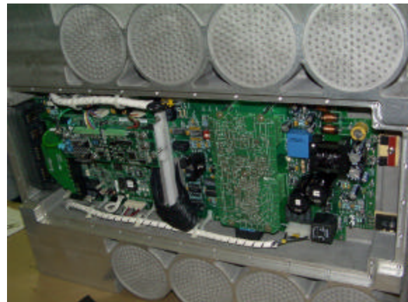
Fig. 8: The bottom side of the package shown in Fig. 6, with the cover removed. The capacitor cooling bays are on the top and the bottom of the photo. Courtesy of Saminco, Inc.
