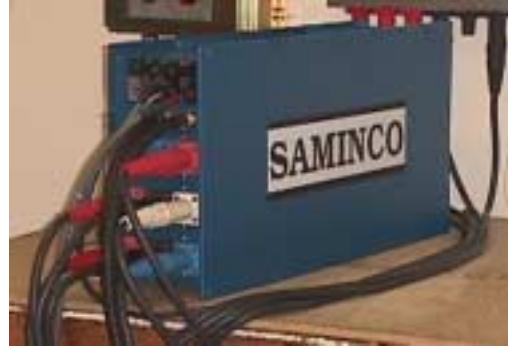
Fig 7: Saminco P4 DC to AC Inverter
